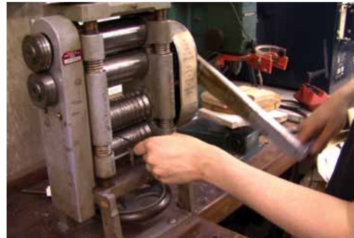
Rolling out the wire
