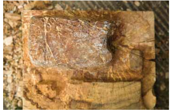
The male part of the mould, or the “plug member”
