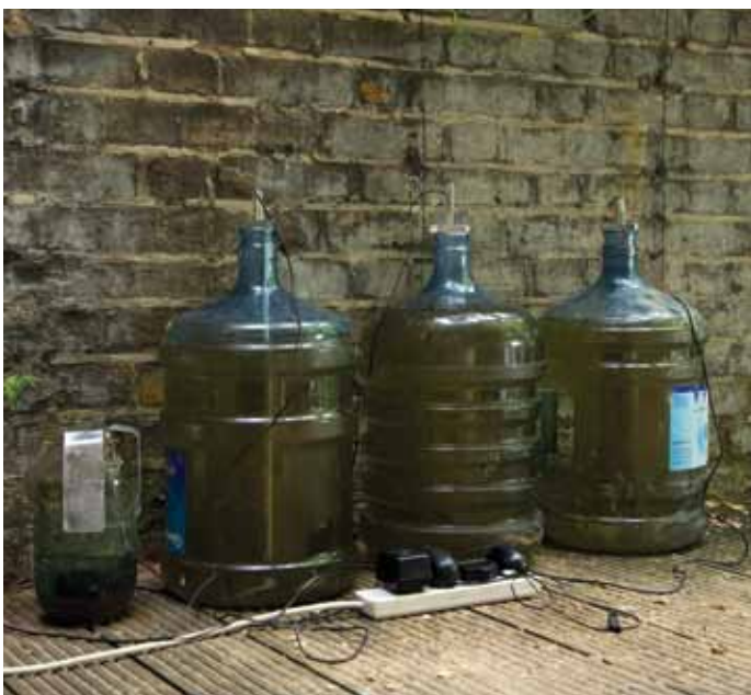
Extracting copper electrolytically
